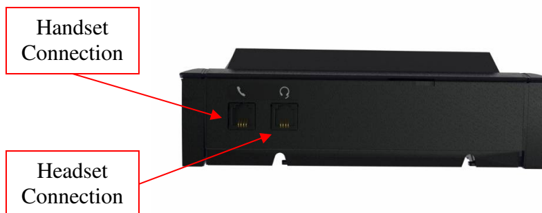
Figure B.4 Speakerbox Rear View – External Audio Device Connections
